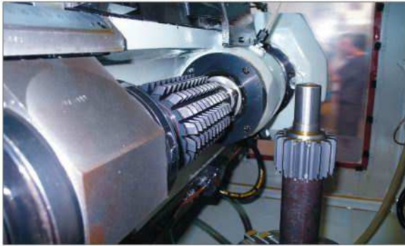
高效数控滚齿机 High efficient digital-controlling gear hobbing machine
