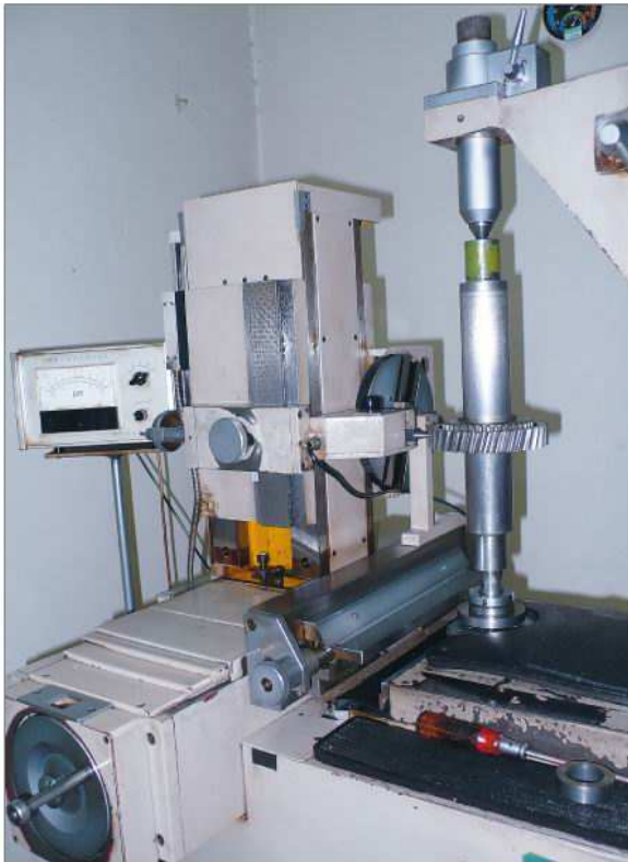
3204B齿形齿向检查仪 3204B checking instrument for gear shape and alignment
